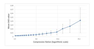
The HUNPCA compression algorithm has been evaluated in terms of data loss according to the similarity metric Spectral Angle Difference (SAD) and the Root Mean Square Error (RMSE). Its performance is compared with the CCSDS 121.0, 122.0 and 123.0 compressors.
